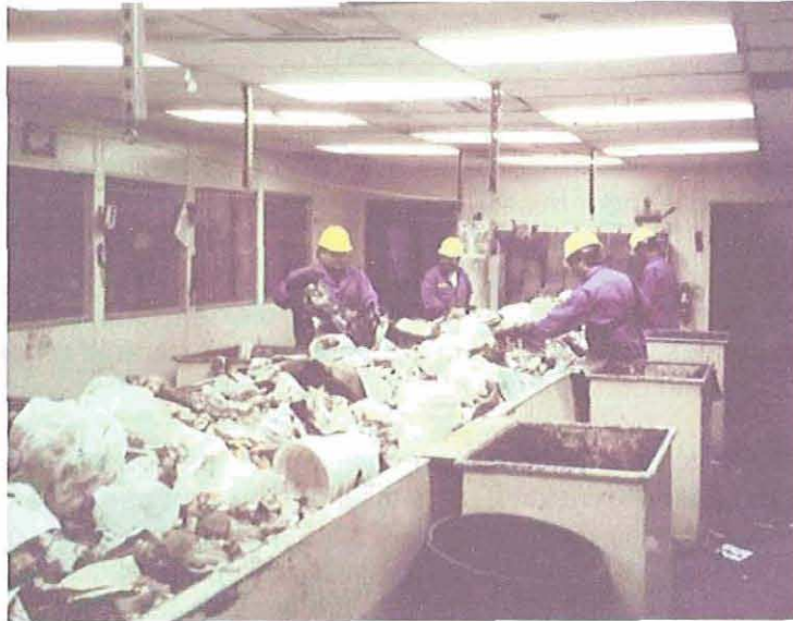
Photo 3-25: Compost sort line at the Rapid City MSW-composting facility The compost-sorting station accommodates six pickers who pick out misplaced recyclables, as well as large, non-degradable items, such as five-gallon buckets, plumbing supplies, etc.
